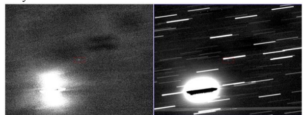
Figure 34. A shift&stack data set of a faint NEO. The stack consists of 31 exposures of 19 seconds duration obtained with the 1.82-m Plaskett telescope of the National Research Council of Canada. The ‘seeing disk’ for the night was 1.8”
