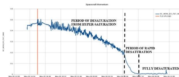
Figure 10 Flight telemetry data showing momentum dumping in NEOSSat's Dipole Desaturation mode. Hyper-saturation is avoided operationally, ensuring rapid desaturation (~ 1 orbit) during routine operations
